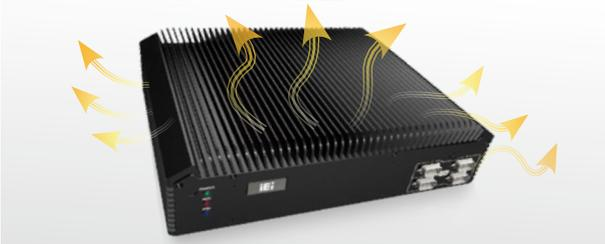
With IEI's fanless solutions, your vessels can avoid the bothersome of replacement of fan, increasing safety and efficiency for the crew and the entire ship.
