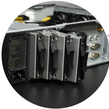
Four hot-swappable HDD/SSD bays with RAID 0/1/5/10 support
