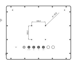
Mechanical 304 Stainless steel chassis(default), 316 Stainless ste Construction chassis(optional) VESA mount 100 x 100, Yoke mount for optional Mounting IP Rating Total IP66/IP69K 470 x 388 x 60 mm Dimensions Net Weight 9.5 kg
