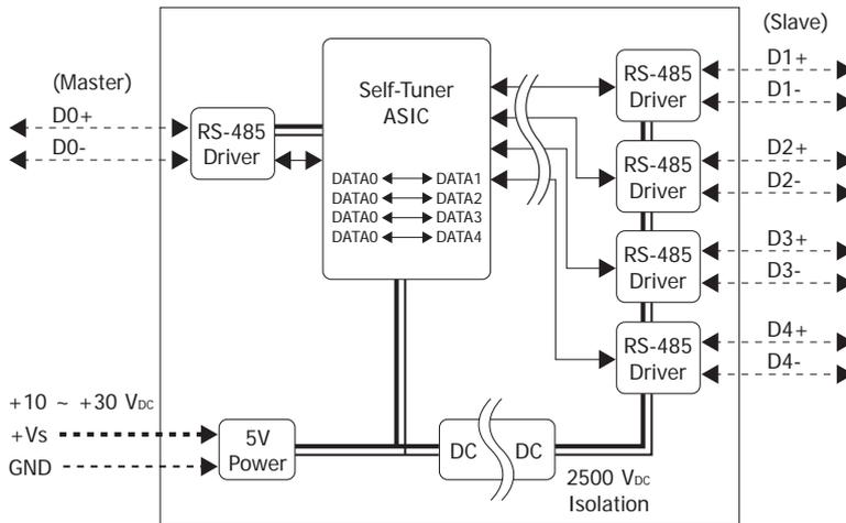
The following block diagram shows how I-7514U was designed as independent channel. Data coming from the master input will be transmitted to all four RS-485 slave channels. But data coming from the slave channels will be returned to the master input only. Thus reduces the possibility of interference between each RS-485 slave loop and makes the RS-485 networks more robust and reliable.
