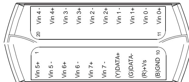
**Wire Connections****I-7017R/M-7017R****Voltage Input Wire Connection**
